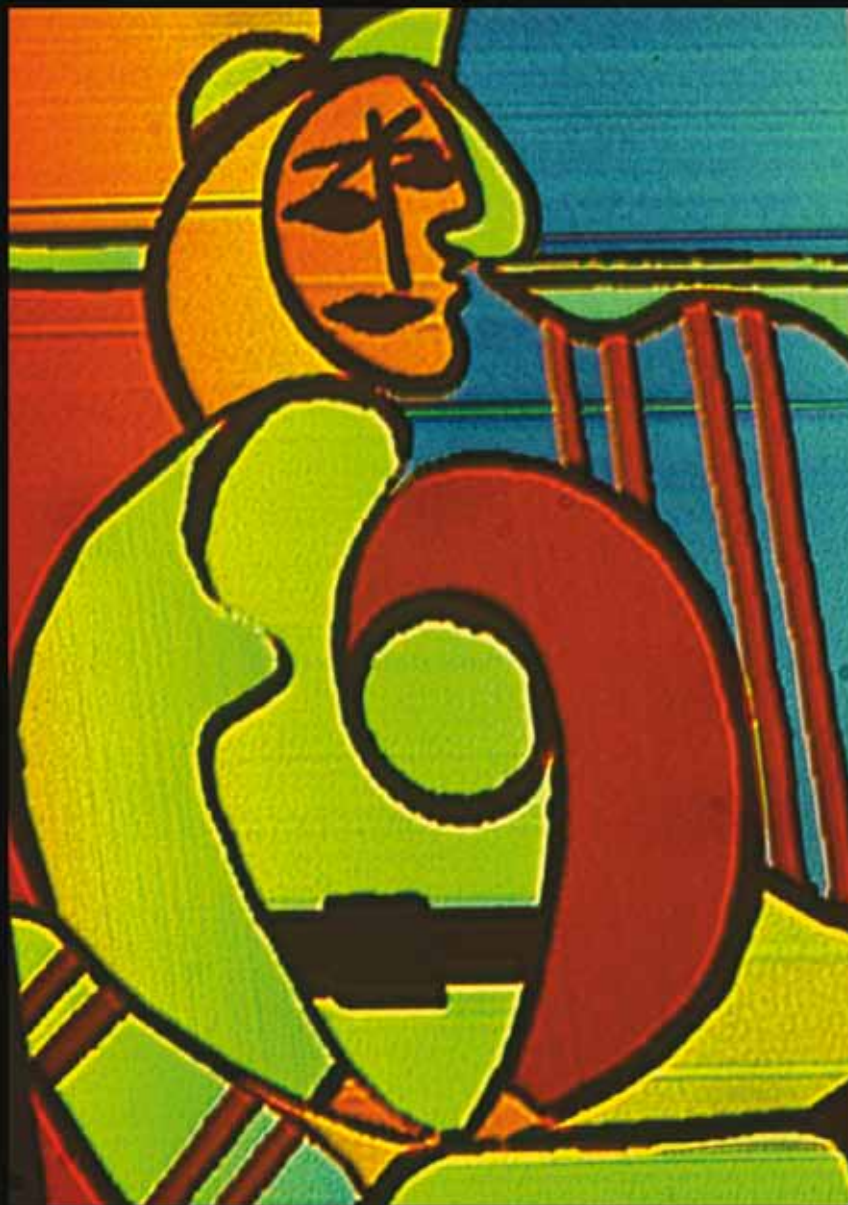
Replica of “The red armchair” by Pablo Picasso in porous silicon Bragg reflectors
