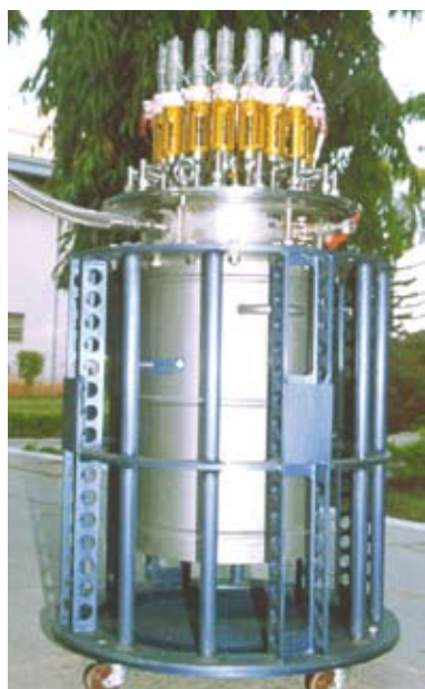
Fig.2. Sampling pod housing the cryoamplifiers carried on a (blue) carriage support.
