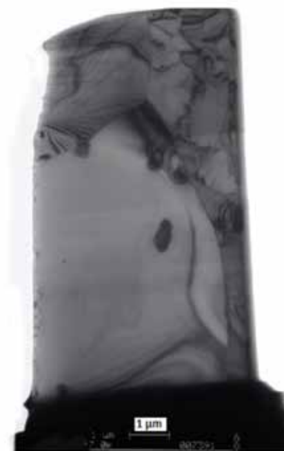
Figure 3: SEM micrograph of TEM foil (5 × 10 μm) of zircaloy prepared by FIB. Thickness less than 80 nm was achieved.
