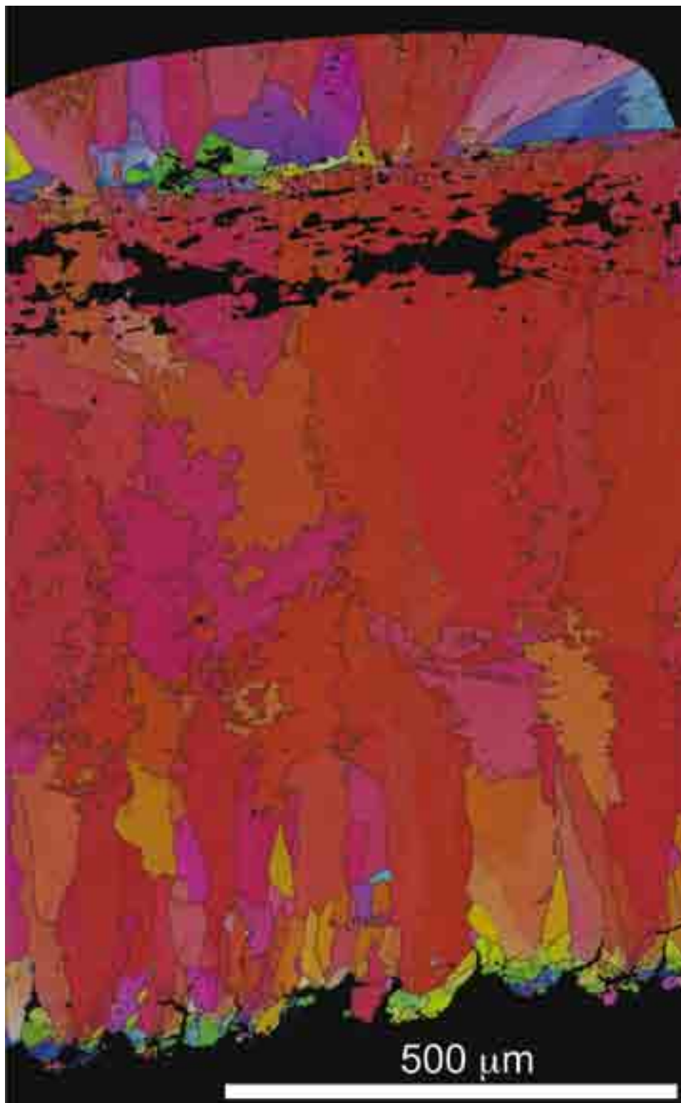
Fig. 10: An EBSD orientation map of a present day emu egg, coloured using the same scheme as in figures 6, 8 and 9. Note a more complex layered structure than seen in the flamingo egg (figure 9) and the fossilised avian example (figure 8). The map was reconstructed from a grid of 746 by 1226 individual EBSD measurements at 1 \mu\text{m} spacing.
