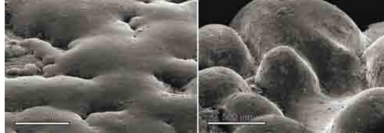
Fig. 2: Secondary electron images taken in the SEM of the exterior surfaces of two eggshells. On the left is a modern day emu egg, on the right is a fossilised Cretaceous titanosaur egg. The sample was tilted to approximately 50° in both cases.
