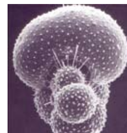
Fig. 4. A shell exhibiting strong line of sight BSE contributions to the image when its surface pointed towards the top right of the display and darker areas shadowed from direct BSE contribution.
