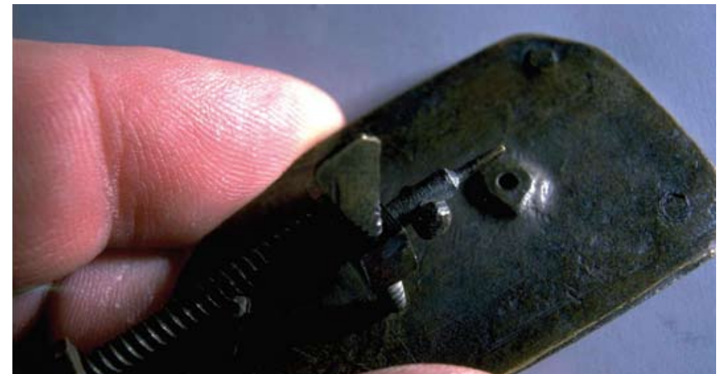
Fig. 7. LEEUWENHOEK MICROSCOPE IN CLOSE-UP. The brass microscope at Antwerp measures 28 x 47 mm and Ford photographed it in close-up to show the details of the stage, focussing and lens assembly. This is No 2 in the microscope collection of the Royal Antwerp Zoological Society and doubts have been raised about its authenticity. It appeared without provenance in the private collection of Dr Henri van Heurck around 1900, which makes its exact origins unclear.
