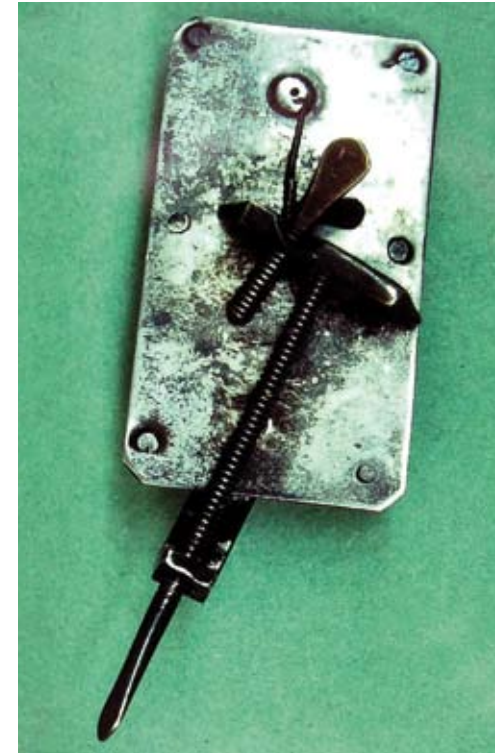
Fig. 6. A SILVER MICROSCOPE FROM MUNICH. Many of the microscopes were made by Leeuwenhoek from silver, which is easier by far to manipulate and shape. This example is in the Deutsches Museum in Munich, Germany, and has a specimen pin made from forged iron. Although not usually published, this is the kind of microscope that Leeuwenhoek bequeathed to the Royal Society. They were still used for critical microscopy into the nineteenth century before being lost.
