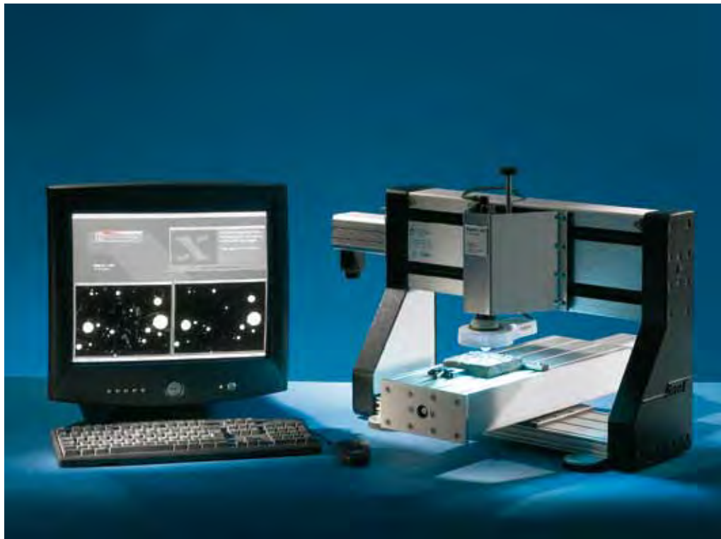
Fig. 4. The RapidAir 457, Automated Air Void Analyzer system for concrete (courtesy of Concrete Experts International).
