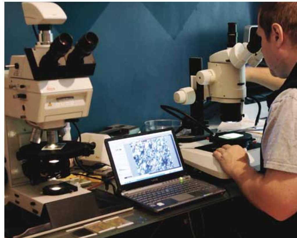
Fig. 2. Microscopical examination using the low-power stereo microscope (right) and high-power petrological microscope (left). Courtesy of IBIS Limited.
