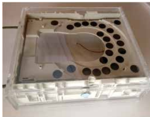
Fig.1. The airtight drawer sampler which was opened and closed by remote control in the stratosphere, showing scanning electron microscope studs onto which stratospheric particles were directly deposited.
