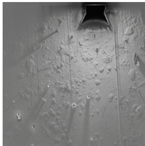
Christopher's favourite image: FIBing the moon' – digging trenches in resin for 3D imaging of cells using Focused Ion Beam SEM.
