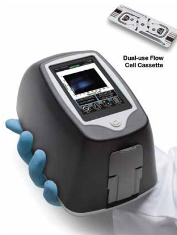
Figure 1 – Orflo Technologies Moxi Flow System and dual-use flow cassette (inset). The Moxi Flow is the World's first flow cytometer to combine the Coulter Principle for precise particle sizing and cell counts with a (single-channel) fluorescence (PMT) measurement for "Assays on Demand", including highly accurate PI-based viability, Annexin V-PE apoptosis, immunolabeling, and RFP transfection efficiency measurements.
