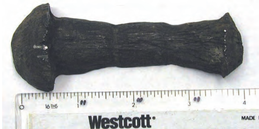
Fig. 1. A macro photo of a hull rivet recovered from the wreck site. It shows a "woody" appearance due to the ferrite being corroded away, leaving ridges of slag. The right end head of the rivet has popped off, leaving the residue of the inside of the head.
