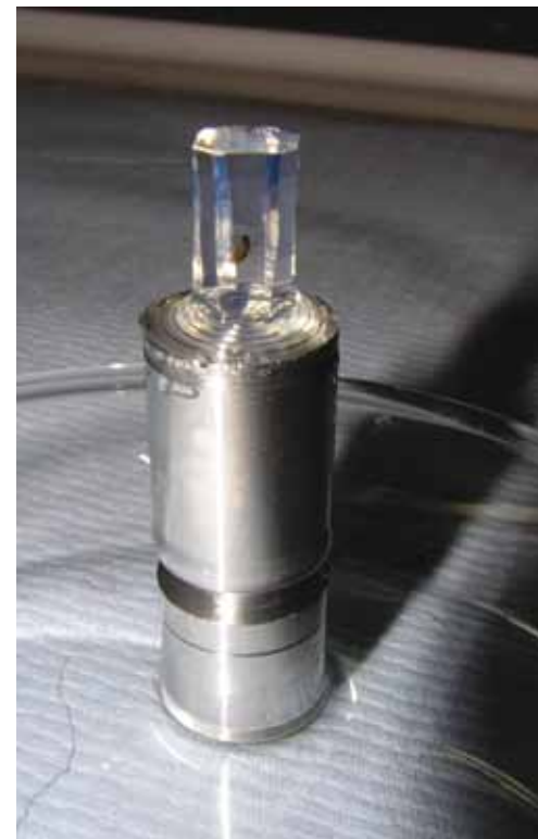
Fig. 2. An agarose block containing a specimen.
