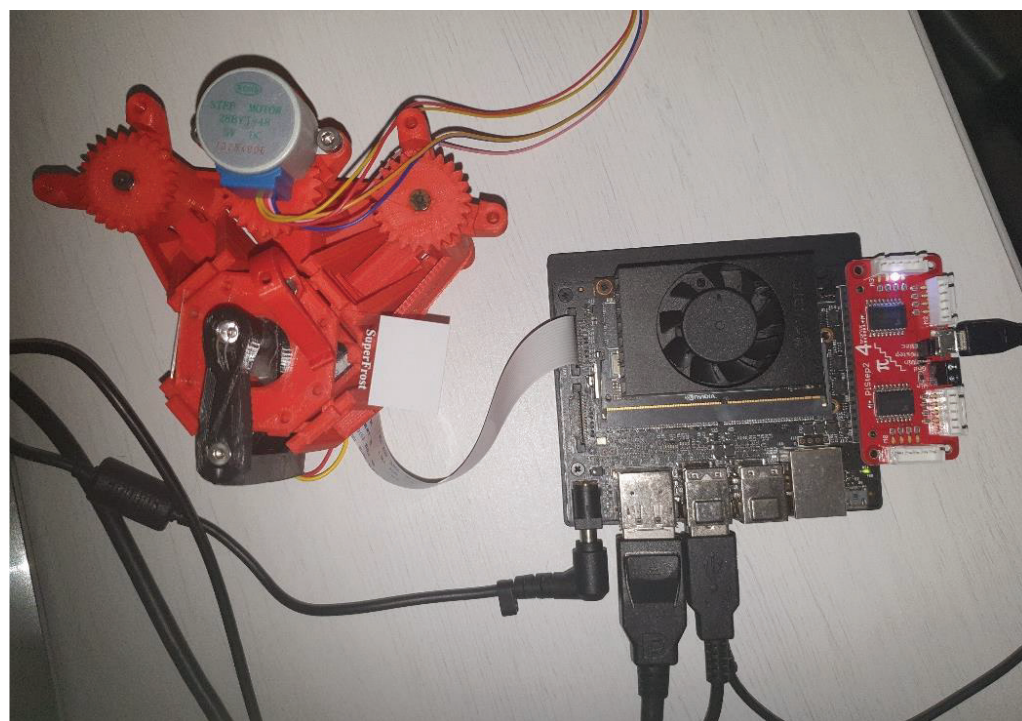
Fig. 1. Image of the experimental setup. The Jetson Xavier NX paired to the 3D printed microscope. The OpenFlexure (left) is 3D printed and can allow for full 3D imaging since it has a moving stage.
