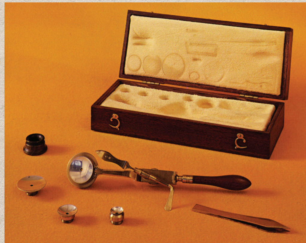
Figure 3. Lieberkuhn – type microscope, 1800
