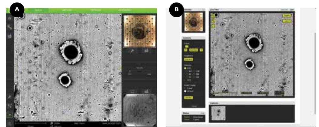
Figure 2: The Open University programmers have taken control of the manufacturer's software operating the microscope (A) and instead created user-friendly web interface (B). The image shows one of the craters from the Stardust Collector that were used for students' projects.
