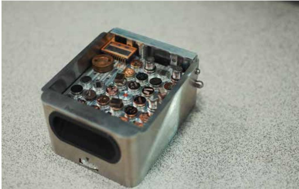
Figure 3: The compact stage of desktop SEM holds samples of up to 10 cm in length, by 10 cm width, by up to 6.5 cm depth.
