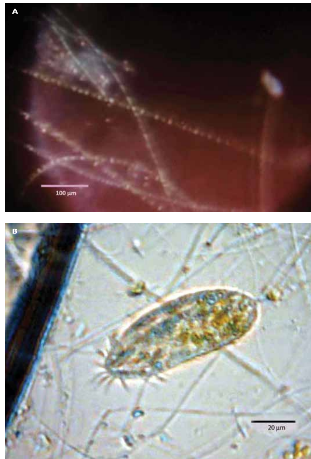
Figure 5. A) Single lenses demand meticulous adjustment. In a BBC television documentary, a replica simple microscope was used to record aquatic microorganisms, though this indistinct result is little improved on what can be perceived with the naked eye. B) A lens magnifying 60x and ground for the author by Es Reid of Cambridge allows us to demonstrate the capacity of a single lens to resolve detail. We can observe the active cirri and cytoplasmic inclusions of an active Stylonicchia grazing among chlorophyte algae.
