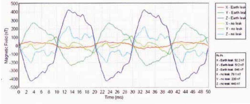
Figure 3. Magnetic fields from earth current leakage.
