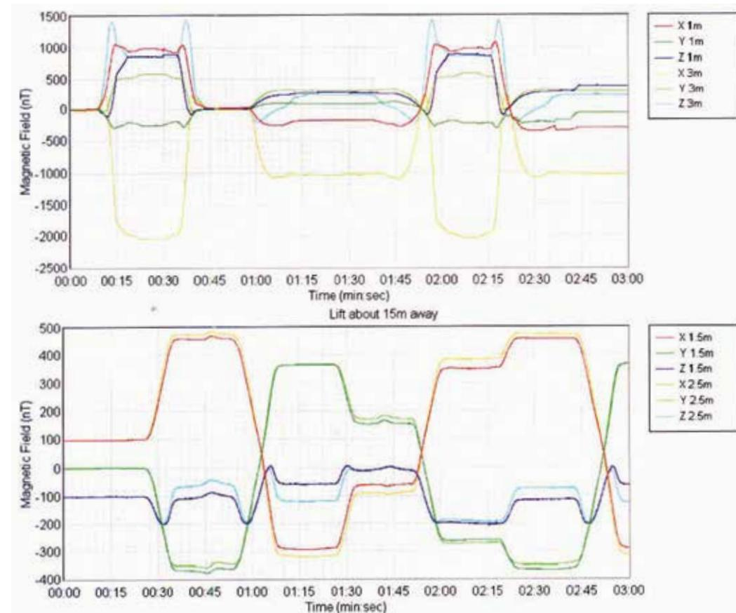
Figure 7. Magnetic fields from lifts.
