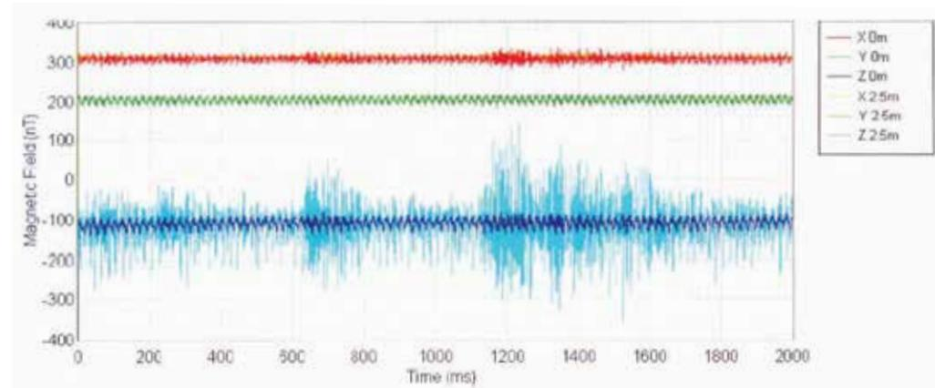
Figure 10. Magnetic fields from hearing loops.
