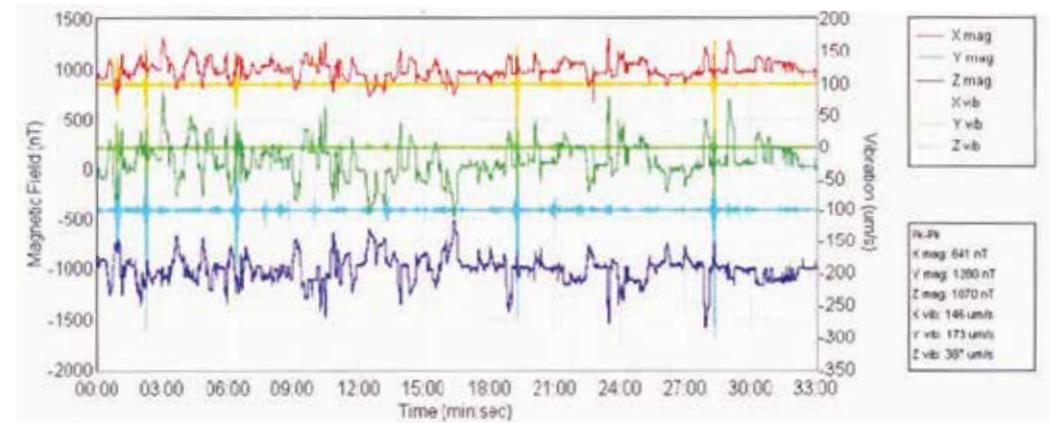
Figure 6. Magnetic fields from trams and trains. The three magnetic axes show how interference from power cables is constantly changing. Vibration bursts can be seen when trains are closest, and demonstrates how magnetic interference can be high when vibration level is low.
