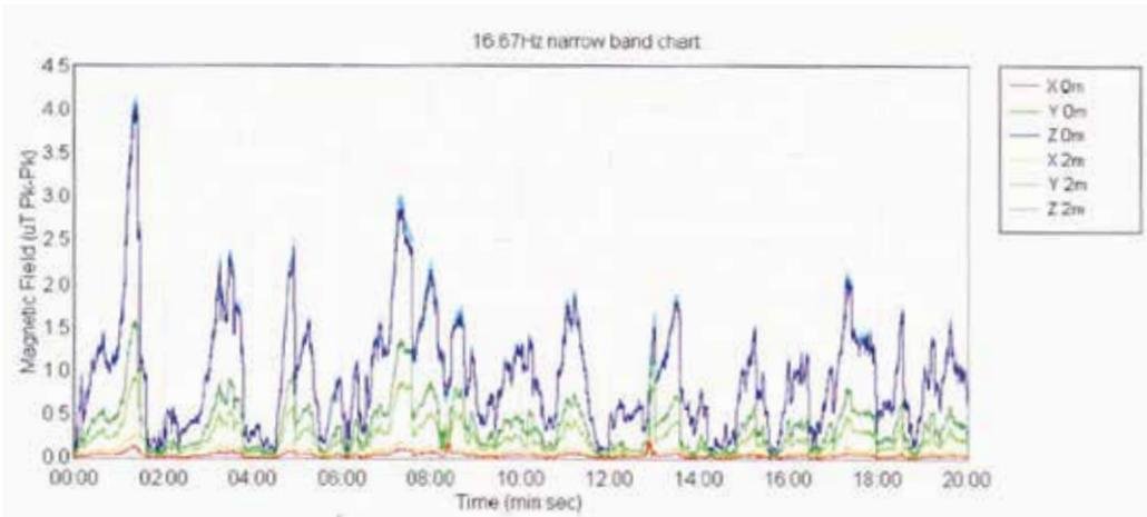
Figure 5A. Magnetic fields from trains. X and Y are the two horizontal axes while Z is the vertical axis. X is parallel to the track in this image.
