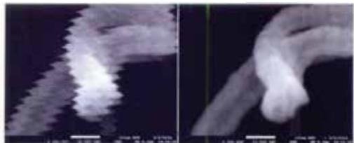
Figure 1B. The effect of a field cancelling system on interference caused by an AC field.
