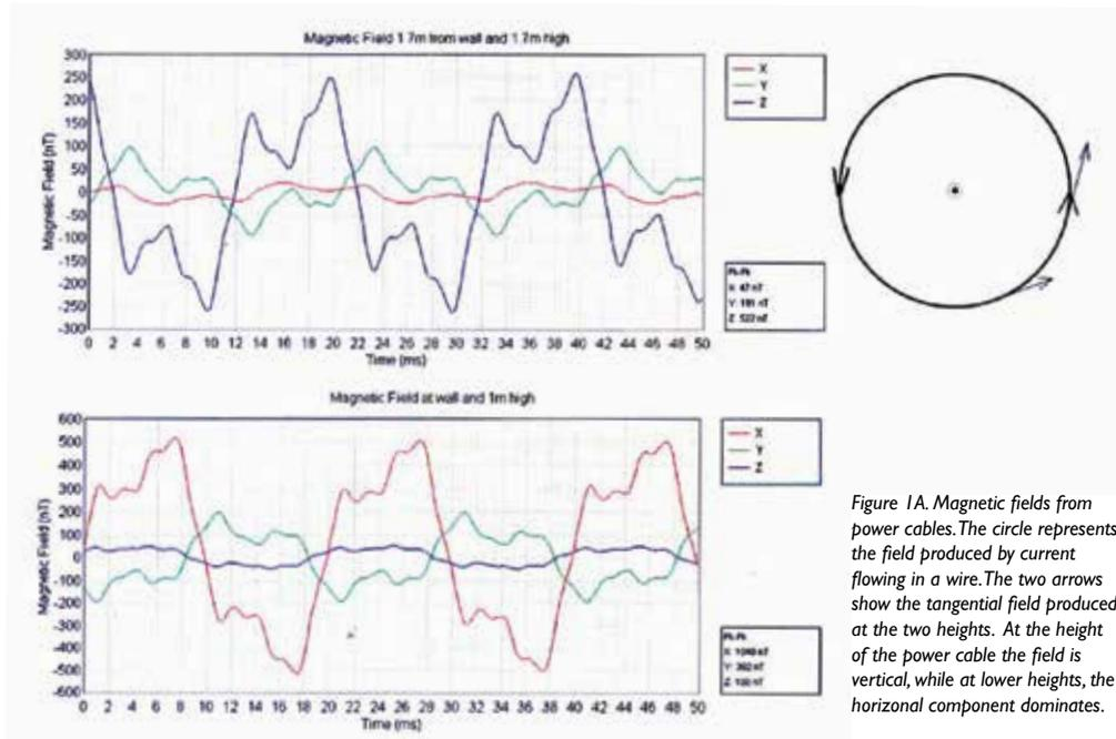
Figure 1A. Magnetic fields from power cables. The circle represents the field produced by current flowing in a wire. The two arrows show the tangential field produced at the two heights. At the height of the power cable the field is vertical, while at lower heights, the horizontal component dominates.
