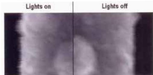
Figure 4. Magnetic fields from lighting. The microscope image on the left was taken with the lights on. The image demonstrates a high level of interference, shown by the jagged edge. This is reduced in the image on the right which was taken with the lights turned off.
