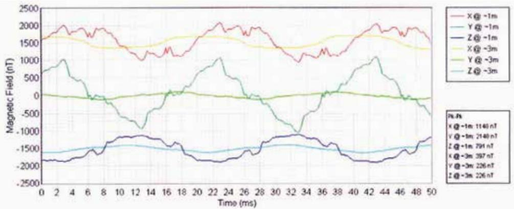
Figure 2. Magnetic fields from distribution boards.
