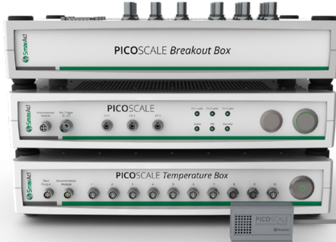
PICO SCALE Controller with accessory components: Breakout Box for convenient access to digital and analog signals, Temperature Box to read up to ten PT1000 temperature sensors, Environmental Module for compensation of air temperature, pressure and relative humidity.
